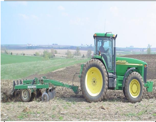
Chiseller (Deep Ploughing , Function: Loosen & Aerated the soil by break hard pans of soil )
