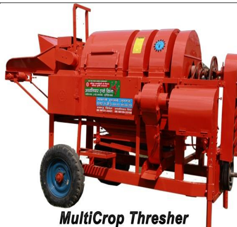
Multi crop thresher (Threshing all type of grains)
